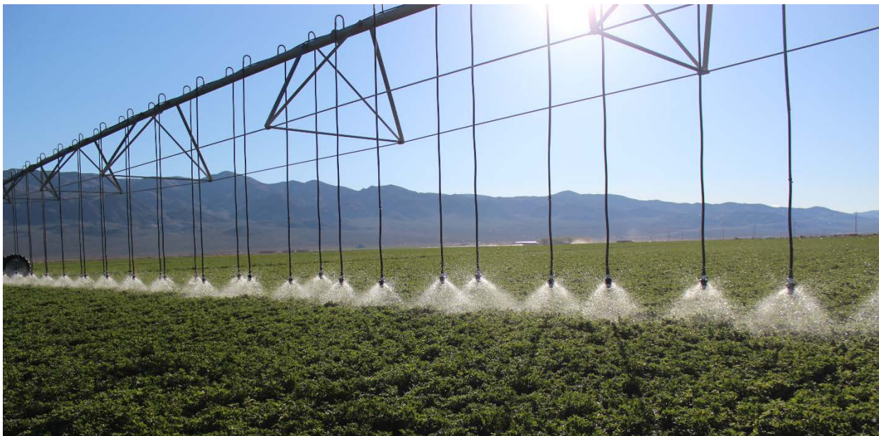
Image 2. LEPA applicators were at close spacing of 30-inches, 18-inch height, with 10-psi pressure regulators.
