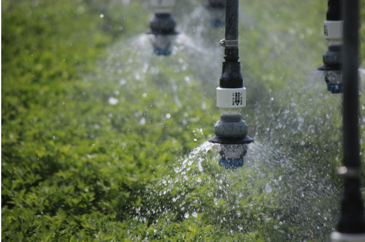
Image 3. LEPA applicators demonstrated increased irrigation efficiency by making more water available for plants.
