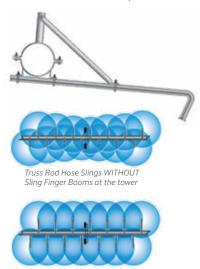
Truss Rod Hose Slings WITH Sling Finger Booms at the tower
