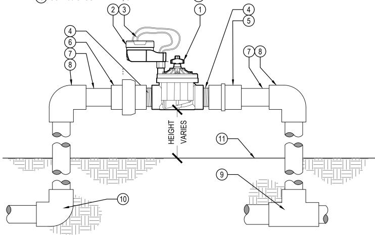
IN-LINE VALVE (ICV) WITH CONTROLLER (SENNODEBT) AND UNION
