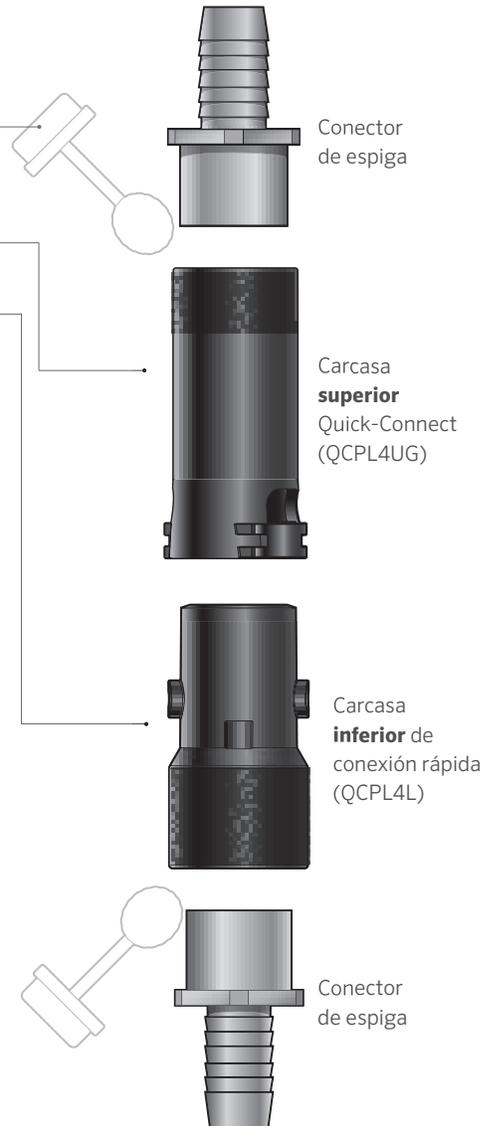
**MONTAJE DEL KIT COMPLETO DE ACOPLADOR QUICK CONNECT (QCPLASM4BRB) EN UN TRAMO DE MANGUERA:**
