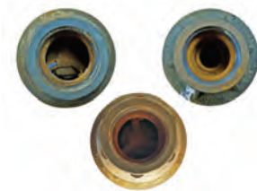
Inlet and outlet of worn pressure regulators.
