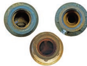
Inlet and outlet of worn pressure regulators.
