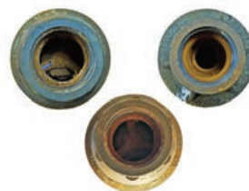
Inlet and outlet of worn pressure regulators.
