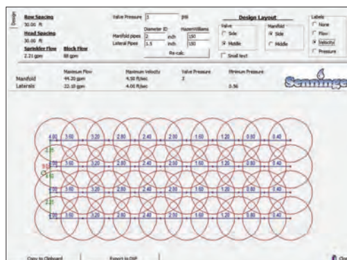
Layout calculator renders sprinkler system designs and provides specifics on flow, velocity and pressures along manifolds in lateral lines.
