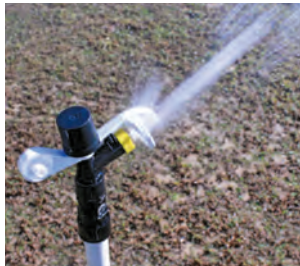
The diffuser distributes some of the flow closer to the sprinkler for better uniformity of application.
