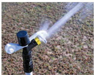
The diffuser distributes some of the flow closer to the sprinkler for better uniformity of application.
