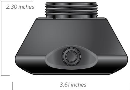
Always be sure the Universal Magnum Weight is tightly threaded into the bottom of the i-Wob®2. 140 inch-lbs. torque recommended.
